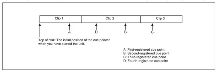
If cue points are registered as shown in the above figure, pressing the NEXT button repeatedly with the \(\frac{1}{2}\) (CUE) button held down makes the cue pointer jump in the order ARBRCRD.
